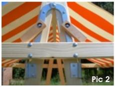
**4.** Put the canvas roll on both Gabel G from back side (hands free & no weight to support!) then unroll till the inner wooden pins are visible. Plug in the pin to the hinges of one end of G and throw the canvas over the top. To fit in the canvas to the other end of G open the wooden locking bolds of both sides on S to allow G to slip out a bit of the hinges - see Pic 2.
